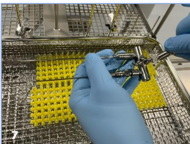
Connect port D to the WD using a silicone tube with a Luer-lock-compatible attachment.
