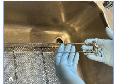
Screw the hollow needle with fine thread onto connection B as far as it will go.
